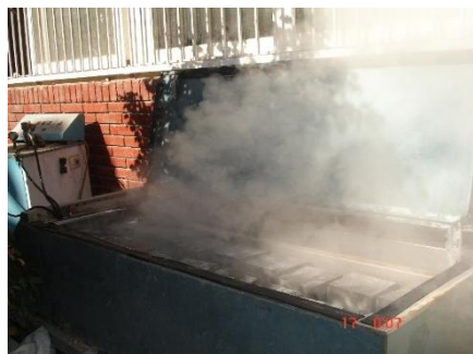
Figure (2), The steam curing tank
