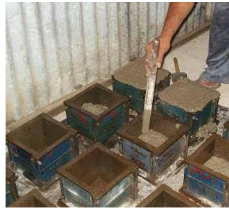
b) compaction of fresh geopolymer concrete
