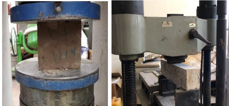
a) Compressive strength test b) Flexural strength test
